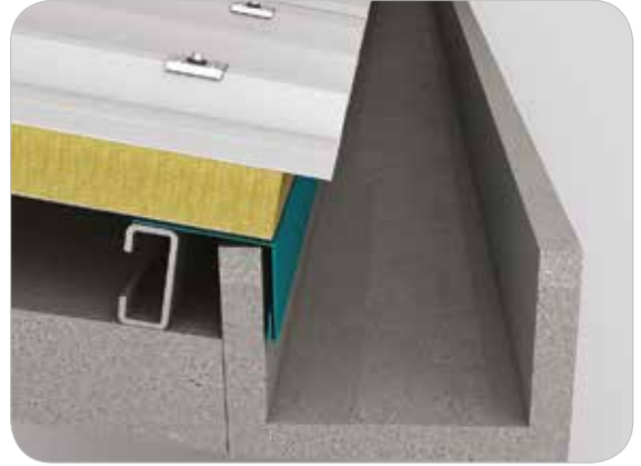
Oluk Betoneme Detay / Gutter Detail
